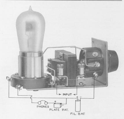
This unit provides a complete audio frequency amplifier unit which may be used with any type of detector set, tube or crystal. Particular attention has been given to the ease of panel mounting. This unit is made in two types. Be sure that the proper unit for your tube is used.
